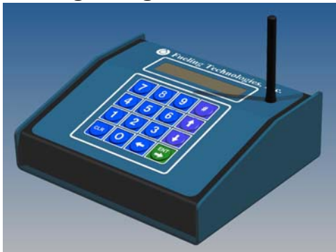
One FTI console can monitor up to thirty tanks
